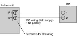
(The wire length between indoor units should be 200 m or less.)
